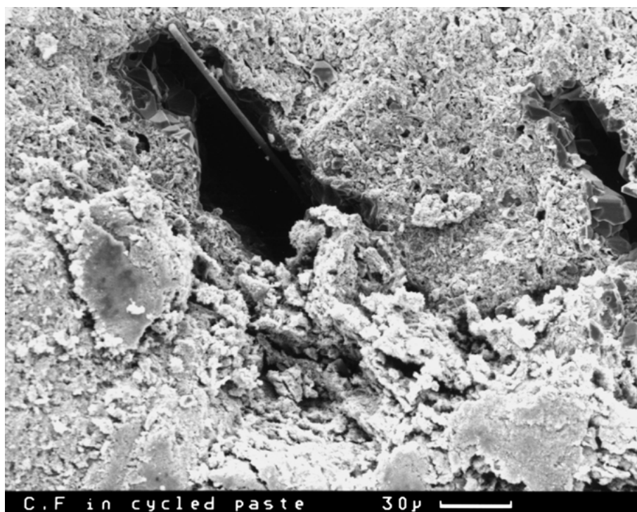
Figure 2 Carbon fibres evident in cycled pastes.
