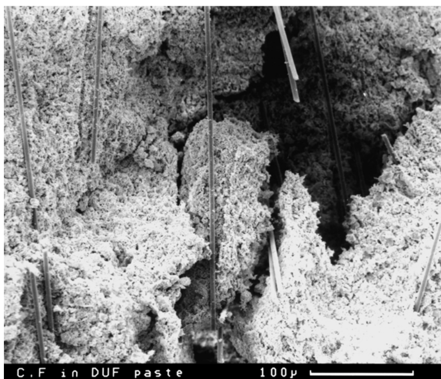
Figure 1 Dried unformed paste containing carbon fibres.
